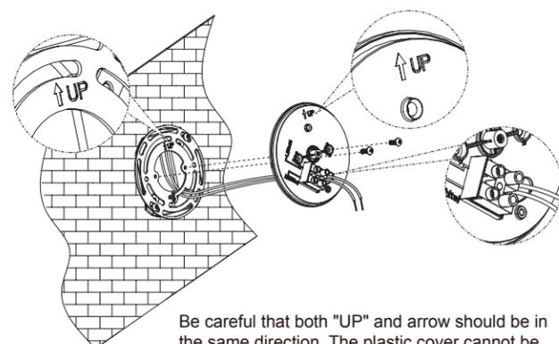
Be careful that both "UP" and arrow should be in the same direction. The plastic cover cannot be rotated to avoid wires damage.
