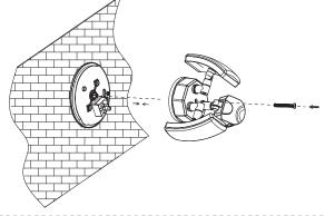
Align the lamp body with plastic cover, tighten the screw through the lamp body, then adjust the sensing center area.
