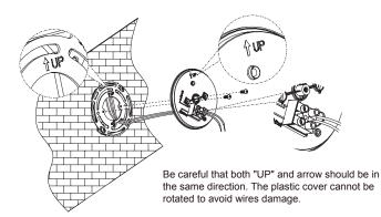
Wires to be pass through the hole of plastic cover. Install the plastic cover to circle crossbar with screws.
