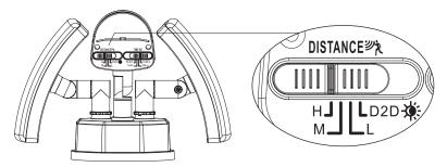
**DUSK TO DAWN FUNCTION:** Select the D2D setting on the distance slider. Lights will be on at dusk/night and auto turn off at dawn/daytime. (Light sensor only in D2D mode.)
