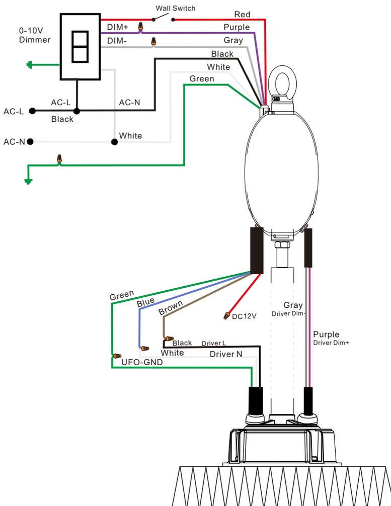
Note: the Emergency Led Drivers Only Work With 0/1-10V Dimmable UFO LED Highbay
