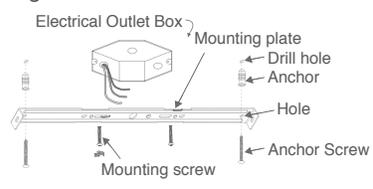
Electrical Outlet Box    Mounting plate
