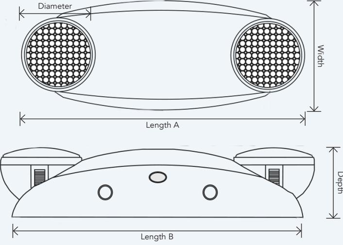
Technical drawing showing the dimensions of the emergency dual light. The drawing includes a top view and a side view. The top view shows two circular light lenses with a diameter of 3.5 inches (88.9 mm). The overall width of the light is 4.56 inches (116 mm). The length of the light is 11.02 inches (280 mm). The side view shows the depth of the light is 2.67 inches (68 mm). The length of the light is 10.15 inches (258 mm).
