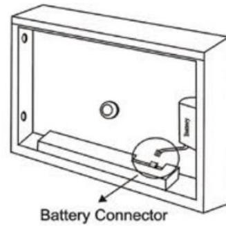
6. Snap fixture onto mounting plate and ensure no wires are pinched. Make sure unit is fully attached.
