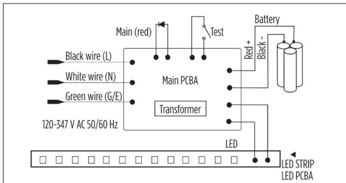
5. Connect the battery to connector on the PCBA.
