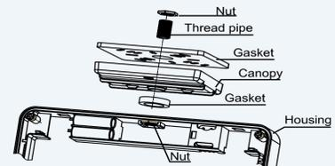
Use provided thread pipe and 2 nut fix canopy on unit, put gasket between unit and canopy.
