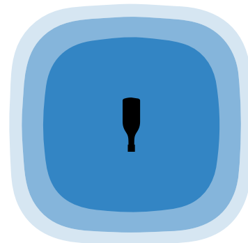
Type III (T3) Light Distribution
